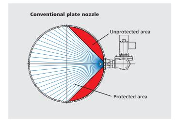
Protected area Should the solenoid valve be damaged or defect, an unintended flow of water may occur. The flow control device integrated into
