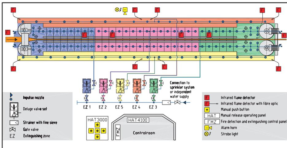
In the past, fire protection for continuous and multi-opening board presses has been less than adequate. Sprinkler systems high above the press are designed to protect the building, but are rarely effective for protection of the Press. The good news is that finally an effective fire protection system has been specifically engineered by Minimax of Germany to protect board Presses and other large objects from fire with relatively little down time or clean-up required.
