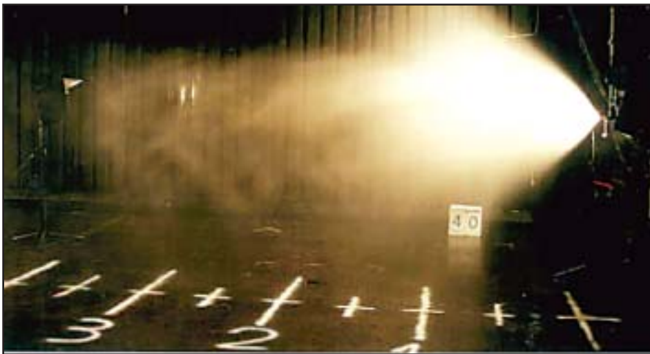
Impulse nozzle spraying (numbers in meters).
