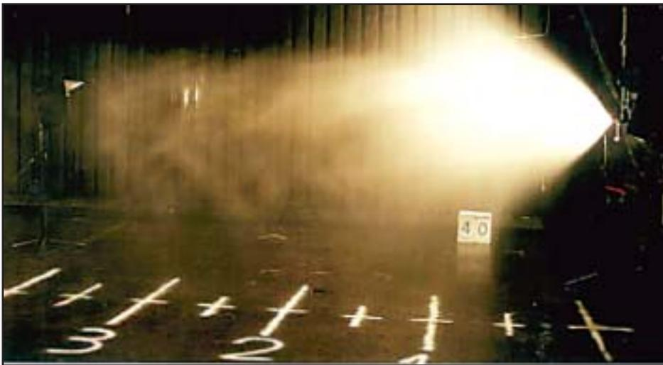
Impulse nozzle spraying (numbers in meters).
