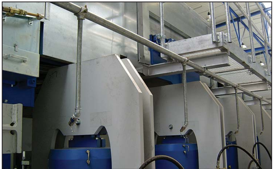
Fine spray nozzles between press frames.
